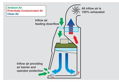
Figure 2. Demonstration on how a Thermo Scientific<sup>™</sup> Class II, Type B2 BSC operates.
